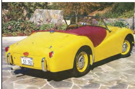
Rear view showing the overriders. The panel on the back where the license plate is mounted holds the spare tire and tools. The most important is for Dzus fasteners used in many places in a TR.
