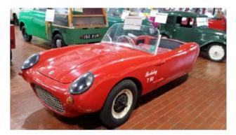
This is a 1959 Berkley Sports SE328. The body is fiberglass and it was powered by a 2 stroke motorcycle engine that propelled the front wheels. There were a total of 1,272 produced.of 5,020. This 3 wheel car was an offshoot of the motorcycle business. BSA produced various models from 1907 until WW II.
