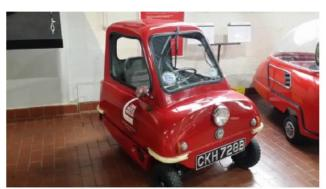
This is a 1964 Peel P-50. This car is recognized as the World's Smallest Production Car. It was priced slightly above a Scooter and had few creature comforts. The 50cc engine is only slightly larger than most Weed Whacker Engines. Since the engine came from a Scooter, it did not have the reverse gear. A handle was added to the back of the car, called a Reversing Handle, which allowed for reversing the car. Fact; you can pack 43 of these in a typical 2 car garage
