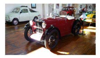
This is a 1932 MG M Type and a total of 3,235 were produced. This was MG's first high volume Sports Car. The typical M Type was Fabric-Bodied, for light weight, however you could get a steel body for an extra money.
