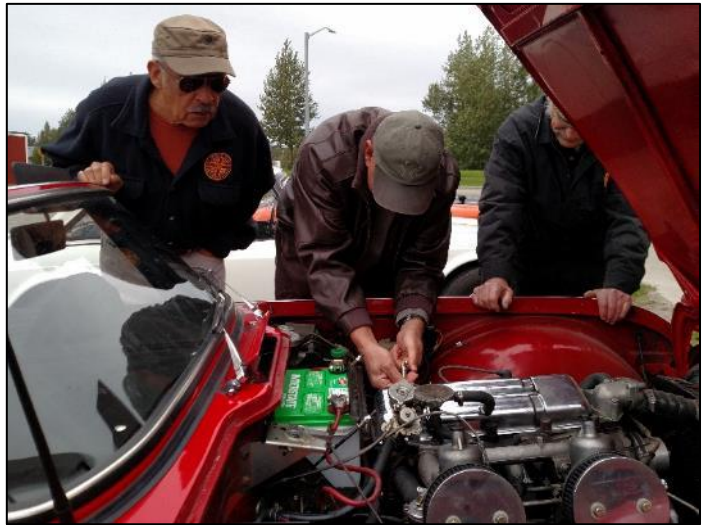
Johnson and Jason help Leonard locate a severe miss. Contrary to the old saying that most carburetor problems are actually in the ignition, this turned out to be a fuel line disconnected from the rear carb.
