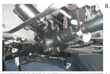
Fit the original mounting clips on the EZ Power Steering column and install this column in the car.
