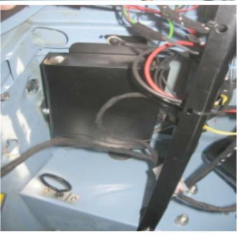
10. Fit the ECU in an appropriate location in the car.
