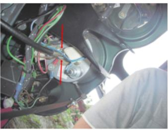
14. If the optional speed adapter is chosen, this can be fixed between the speedometer and cable. Connect the wires of the adapter through the plug with the corresponding colors to the EZ Power Steering wiring loom.
