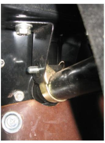
5. Remove the lower mounting bolt from the original steering column.
