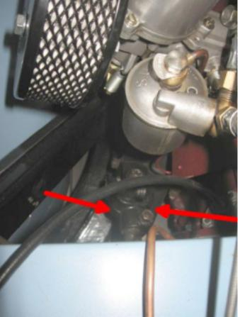
9. Attach the U-joint with the mounting bolt back to the column.
