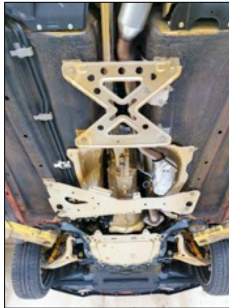
Dry-ice media blasted to clean it completely and prepare all surfaces for the application of the HoneySeal wax to all components and surfaces except for the muffler and catalytic converter.
