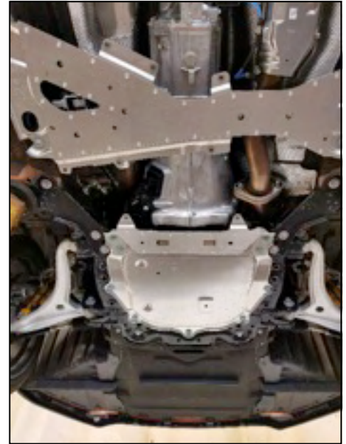
The front is still relatively clean underneath with factory undercoating. Aluminum front suspension arms, black painted steel rear suspension arms, and exposed metal (steel or aluminum) bolts and braces.
